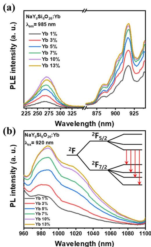
Fig. 4 (a) Excitation ( $\lambda_{em} = 985$  nm), and (b) emission ( $\lambda_{ex} = 920$  nm) spectra of  $\text{NaY}_9\text{Si}_6\text{O}_{26}:\text{Yb}^{3+}$  phosphors with varying concentrations of  $\text{Yb}^{3+}$  ions in NIR region.
