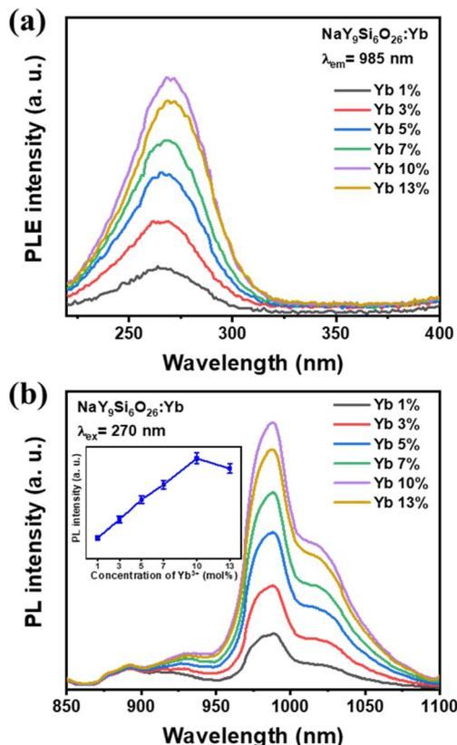
Fig. 3 (a) Excitation ( $\lambda_{\text{em}} = 985 \text{ nm}$ ), and (b) emission ( $\lambda_{\text{ex}} = 270 \text{ nm}$ ) spectra of  $\text{NaY}_9\text{Si}_6\text{O}_{26}:\text{Yb}^{3+}$  phosphors with varying concentrations of  $\text{Yb}^{3+}$  ions.
