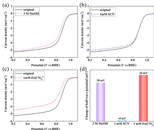
Fig. 5 LSV curves for FeNC-24 in a 0.1 M  $O_2$ -saturated KOH solution at 1600 rpm with (a) 3 M methanol, (b) 1 mM  $SCN^-$ , and (c) 1 mM  $Fe(CN)_6^{3-}$ ; (d) histogram of the change in the half-wave potential.
