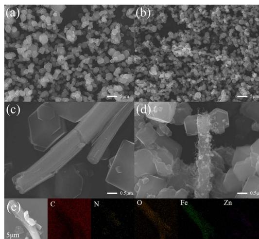
Fig. 1 SEM images of FeZIF-2-0.5Fe (a, c) and FeNC-2-0.5Fe (b, d) and (e) EDS-mapping images of FeZIF-2-0.5Fe.
