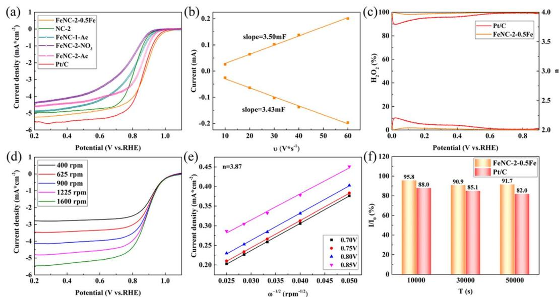
Fig. 4 (a) LSV curves of different catalysts in a 0.1 M  $\text{O}_2$ -saturated KOH solution at 1600 rpm. (b) The fitted ECSA for FeNC-2-0.5Fe. (c) Productivity of  $\text{H}_2\text{O}_2$  and electron transfer numbers of FeNC-2-0.5Fe and Pt/C. (d) LSV curves of FeNC-2-0.5Fe at different rotating speeds. (e) FeNC-2-0.5Fe data fit with the K–L equation. (f) The histogram of the current attenuation rate for FeNC-2-0.5Fe and Pt/C during the CA test.
