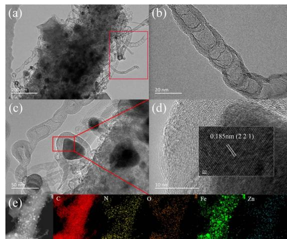
Fig. 2 TEM images of FeNC-2-0.5Fe (a–c); HR-TEM image of FeNC-2-0.5Fe, where the lattice distance corresponds to that in PDF#35-0772; (d) HAADF-STEM and (e) EDS-mapping images of FeNC-2-0.5Fe.
