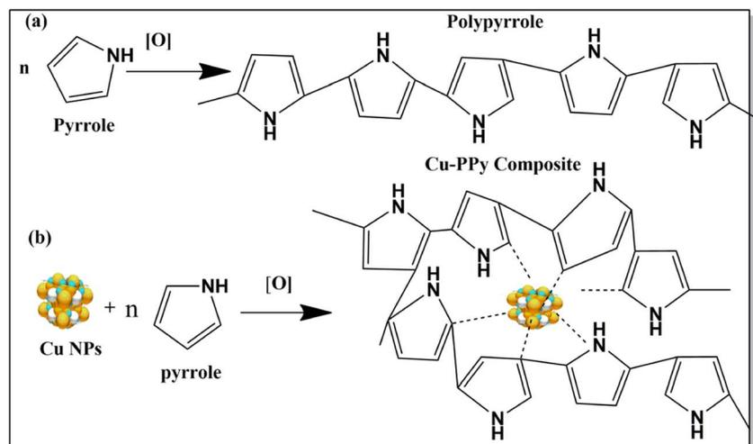
Scheme 1 (a) Formation of polypyrrole (PPy) in the presence of an oxidizing agent (ammonium persulfate). (b) Formation of polypyrrole incorporated around Cu NPs dispersed in pyrrole. Dotted lines show the interaction between  $\pi$  electrons, N–H, and copper NPs.
