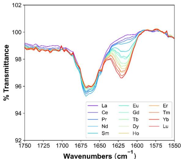
Fig. 5 FT-IR spectra, highlighting the carbonyl stretch for a modifier-free system with 0.04 M TODGA in *n*-dodecane after contact with Lns.
