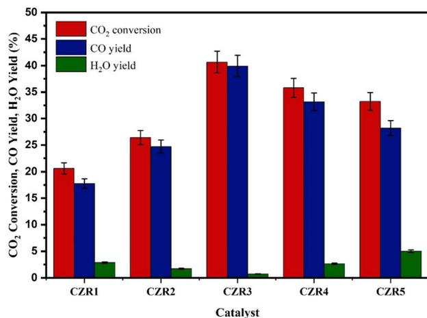
Fig. 11 The CO<sub>2</sub> conversion, CO yield, and H<sub>2</sub>O yield in the reverse water gas shift reaction over various Cu/Zn ratios supported on RSBE. Catalytic reverse water gas shift reaction conditions: temperature = 200 °C; H<sub>2</sub>/CO<sub>2</sub> = 3; pressure = 3 MPa; residence time = 4 h; catalyst weight = 1.0 g.
