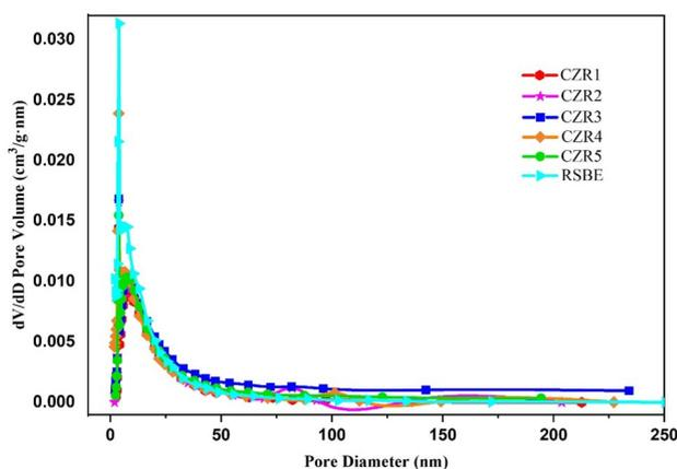
Fig. 8 BJH pore size distribution of reduced catalysts.
