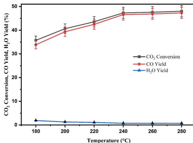
Fig. 12 Effect of reaction temperature on CO<sub>2</sub> conversion, CO yield and H<sub>2</sub>O yield over CZR3 catalyst.
