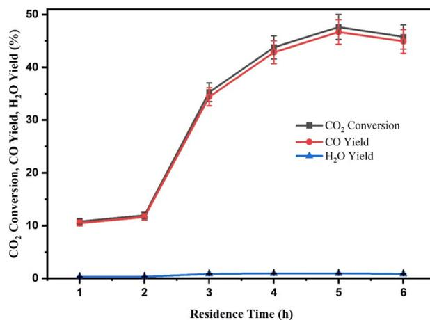
Fig. 14 Effect of residence time on CO<sub>2</sub> conversion, CO yield, and H<sub>2</sub>O yield over CZR3 catalyst.
