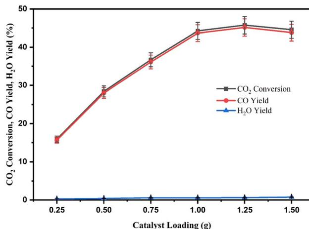
Fig. 15 Effect of catalyst loading on CO<sub>2</sub> conversion, CO yield and H<sub>2</sub>O yield over CZR3 catalyst.
