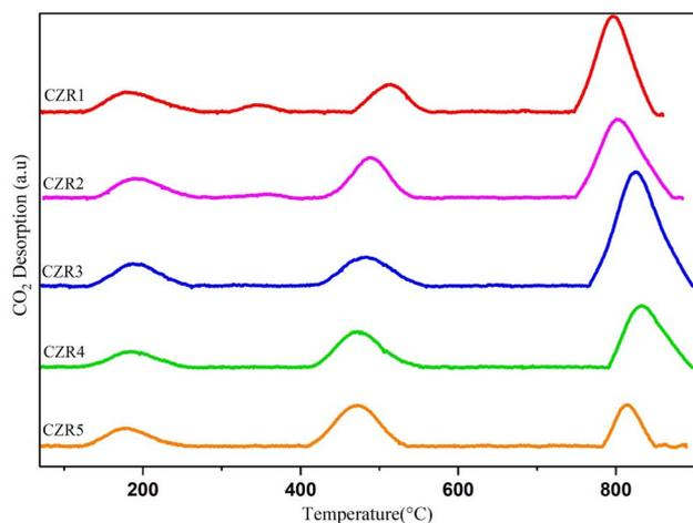
Fig. 6 TPD- $\text{CO}_2$  analysis of reduced catalysts.
