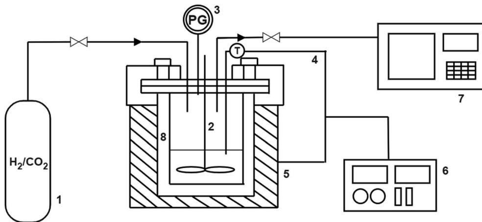
Fig. 1 Schematic diagram of CO<sub>2</sub> hydrogenation experimental setup: (1) H<sub>2</sub>/CO<sub>2</sub> tank; (2) stirrer; (3) pressure gauge; (4) thermocouple; (5) heater; (6) temperature and motor controller; (7) GC; (8) reactor.
