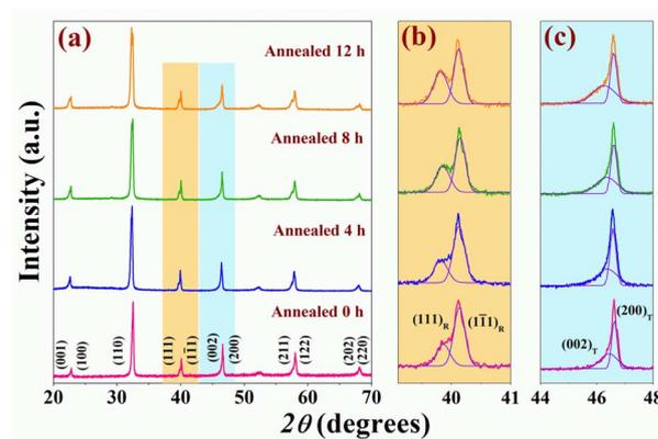
Fig. 1 X-ray diffraction patterns of the BNKT/0.01ZnO ceramics annealed at 950 °C with different annealing times, where (a)  $2\theta = 20\text{--}70^\circ$  (b)  $2\theta = 39\text{--}41^\circ$ , and (c)  $2\theta = 44\text{--}48^\circ$ .
