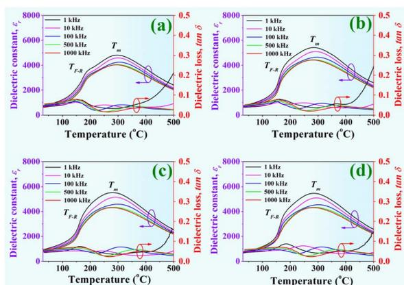
**Fig. 5** Temperature dependence on dielectric constant ( $\epsilon_r$ ) and dielectric loss ( $\tan \delta$ ) of the poled BNKT/0.01ZnO ceramics annealed at 950 °C with different annealing times, measurement at various frequencies from 1–1000 kHz, where (a) 0 h, (b) 4 h, (c) 8 h, and (d) 12 h.
