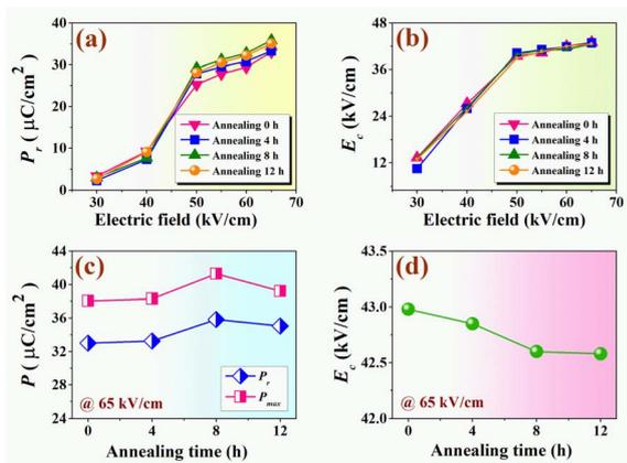
**Fig. 9** Plots of (a)  $P_r$ , (b)  $E_c$  values as a function of electric fields from 30–65  $\text{kV cm}^{-1}$ , (c)  $P_r$  and  $P_{\max}$  as a function of annealing time @  $E = 65 \text{ kV cm}^{-1}$ , and (d)  $E_c$  as a function of annealing time @  $E = 65 \text{ kV cm}^{-1}$  of the BNKT/0.01ZnO ceramics annealed at 950 °C with different annealing times.
