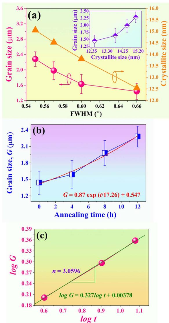
Fig. 4 Plots of (a) FWHM versus grain size and crystallite size (inset shows a relation between grain size and crystallite size), (b) grain size as a function of annealing time, and (c)  $\log G$  as a function of  $\log t$ .
