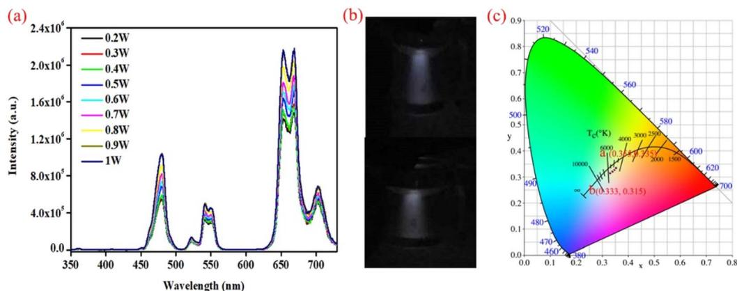
Fig. 4 PL spectra of the UNCPs (sample 3) under 980 nm excitation with different excitation powers (a). Digital camera photographs of the UNCPs, which present white emission under different excitation powers (0.2 and 1 W) of 980 nm excitation (b), and the corresponding CIE coordinates for different excitation powers (0.2–1 W, (c)).
