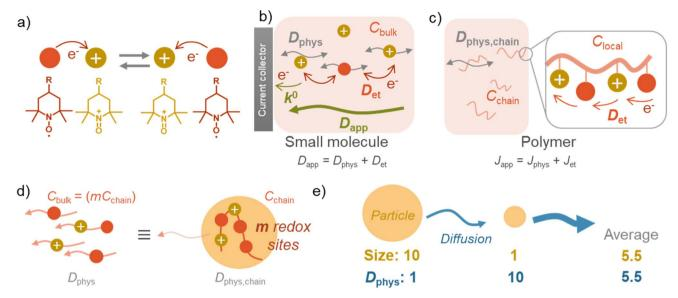
Fig. 2 Scheme of charge transfer. (a) Electron self-exchange reaction by redox-active species, such as TEMPO. (b) Charge diffusion by small molecules. (c) Charge diffusion by polymers. (d) Approximation of a redox-active polymeric chain as small molecules. (e) Scheme of charge diffusion by two particles. Their average diffusion coefficient is 5.5, which never matches the value derived from average radii: 10/(average radii) = 10/5.5 = 1.8.
