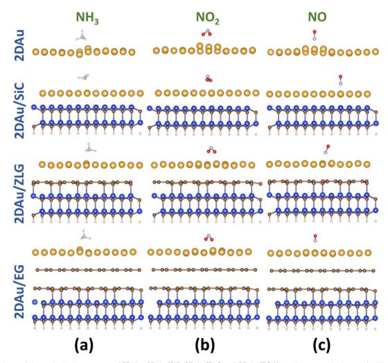
Fig. 7 Side views of the optimized structures of 2D Au, 2D Au/SiC, 2D Au/ZLG and 2D Au/EG (from the top to the bottom) with adsorbed gas molecules: (a)  $NH_3$ , (b)  $NO_2$ , and (c)  $NO_2$ , respectively. Blue, brown, yellow, whitish, pale blue and red balls designate Si, C, Au, H, N and O atoms, respectively.
