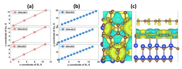
Fig. 2 Mutual dependences of cartesian coordinates of aligned Si and Au atoms for three considered structures: (a) x-axis and (b) y-axis. (c) Charge distribution at EG/ZLG/SiC interface (top and side views). Dashed circles designate the positions of sp<sup>3</sup>-bonded carbon atoms of ZLG. The iso-surface level was set to  $8 \times 10^{-4}$  e Å<sup>-3</sup>. Yellow and cyan colors correspond to positive (charge accumulation) and negative (charge depletion)  $\Delta \rho$ .
