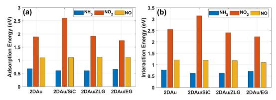
Fig. 8 Comparative bar charts of (a) adsorption energy of gas molecules on different surfaces and (b) interaction energy between gas molecules and gold monolayer, respectively.
