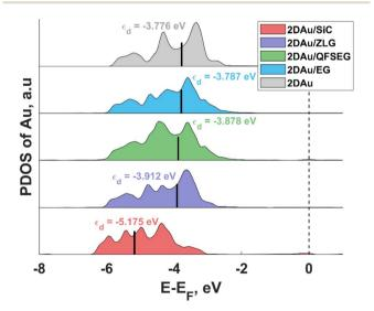
Fig. 6 The projected d band density of states (DOS) for gold in 2D Au, 2D Au/SiC, 2D Au/ZLG, 2D Au/QFSEG and 2D Au/EG systems. Short black vertical lines designate the position of d band centre. The Fermi level is set to zero and indicated by the black dashed line.
