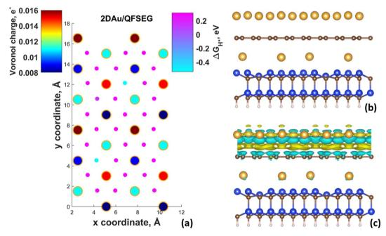
Fig. 5 (a) Map of predicted free energy adsorption,  $\Delta G_{H^*}$ , for the Volmer step on different 2D Au/QFSEG. Small circles correspond to  $\Delta G_{H^*}$  values for H adsorbates at different sites. Large circles represent magnitudes of Voronoi charge on Au atoms belonging to 2D Au layer. Optimized structure of 2D Au/QFSEG (a) and corresponding 3D-CDD (c). The iso-surface level was set to  $5 \times 10^{-4}$  e Å<sup>-3</sup>.
