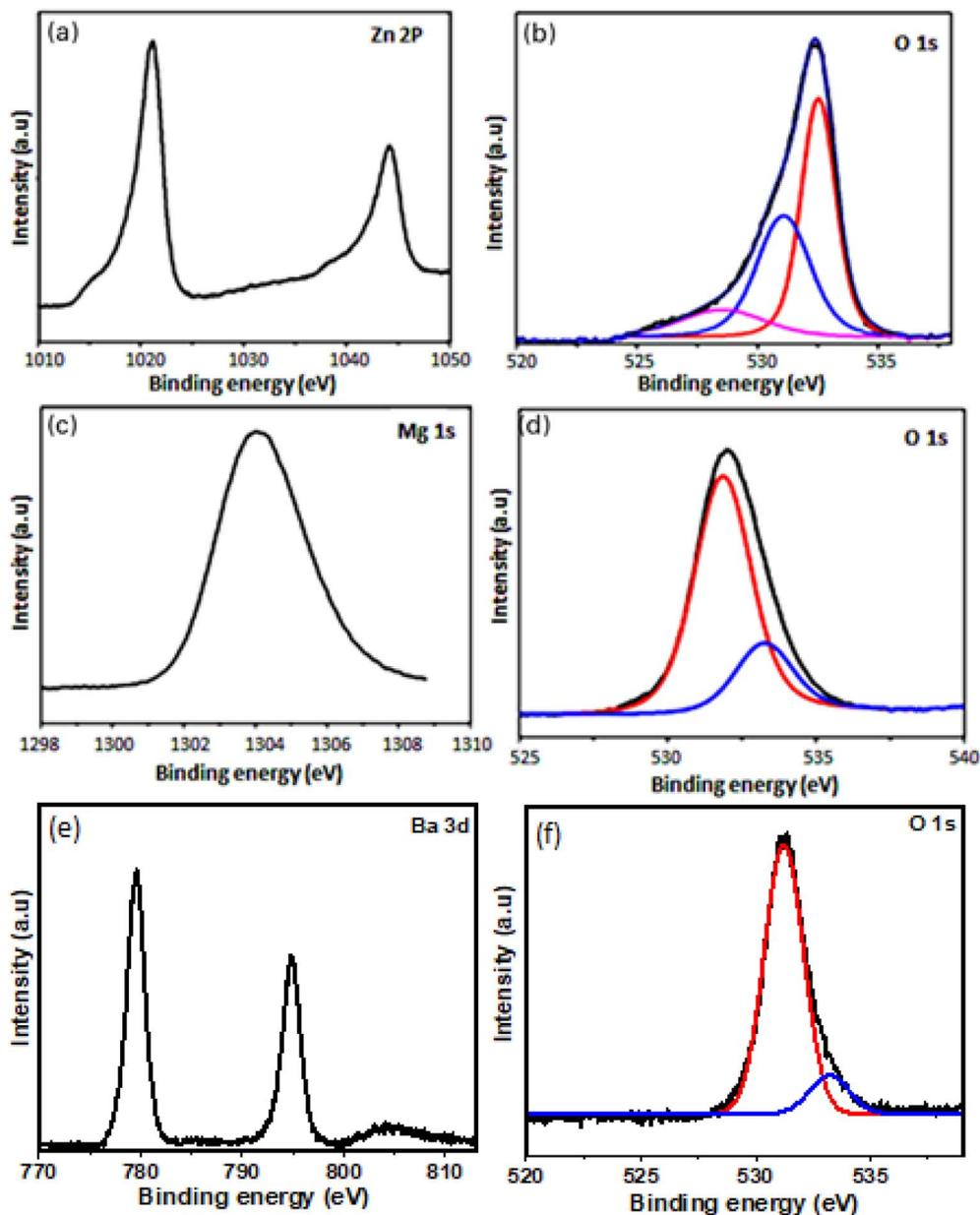
Fig. 4 X-ray photoelectron spectra of (a) Zn 2p (b) O 1s of ZnO<sub>2</sub> (c) Mg 2p (d) O 1s of MgO<sub>2</sub> (e) Ba 3d (f) O 1s of BaO<sub>2</sub>.
