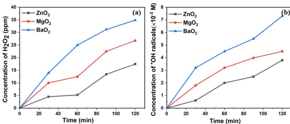
Fig. 5 (a) H<sub>2</sub>O<sub>2</sub> produced (b) ·OH radicals produced by metal peroxides under UV light.
