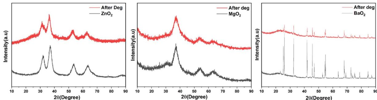
Fig. 10 XRD patterns of metal peroxides after 3 cycles of photocatalytic degradation of dyes under UV light.
