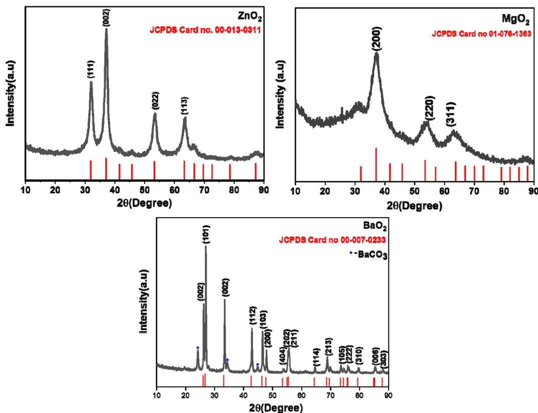
Fig. 1 Powder X-ray diffraction patterns of ZnO<sub>2</sub>, MgO<sub>2</sub> and BaO<sub>2</sub>.
