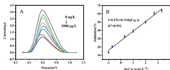
Fig. 9 (A) DPV curves of SPCE/GR/AChE/Nafion sensors in PBS solution (pH = 7.5) containing 1 mM ATCl after being inhibition by different concentrations of ICP for 10 min. ICP concentrations: 0, 0.1, 0.2, 2, 10, 100, 500, 2000  $\mu\text{g L}^{-1}$ ; (B) calibration curve of the inhibition rate of DPV peak current of SPCE/GR/AChE/Nafion sensor versus the logarithmic value of ICP concentration.
