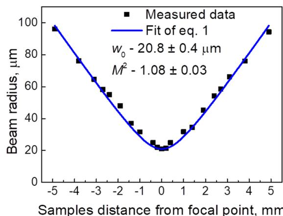
Fig. 3 Laser beam radii at different sample  $z$  positions. Black squares represent experimental data, and the blue line represents the fit of equation. The received parameters were beam waist  $w_0$  ( $20.8 \pm 0.4 \mu\text{m}$ ) and beam quality parameter  $M^2$  ( $1.08 \pm 0.03$ ).
