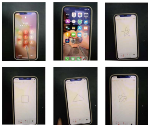
Fig. 10 Hydrogel is assembled into a touch electronic pen, which can unlock the phone.
