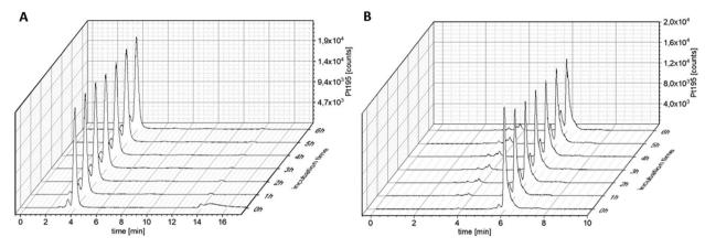
Fig. 5 195 Pt-traces of incubation of 100 µM (A) OxAsaMal and (B) OxAsaOAc in FCS (containing 150 mM phosphate buffer, pH = 7.4) at 37 °C over 6 h, measured with SEC-ICP-MS.
