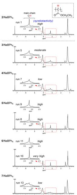
Fig. 2 <sup>1</sup>H NMR spectra of polyEDA's obtained with 2/NaBPh<sub>4</sub>, 3/ NaBPh<sub>4</sub> (run 5 in Table 1), 4/NaBPh<sub>4</sub> (run 7 in Table 1), 5/NaBPh<sub>4</sub> (runs 8 and 9 in Table 1), 6/NaBPh<sub>4</sub> (runs 10 and 11 in Table 1), and 7/NaBPh<sub>4</sub> (run 13 in Table 1), recorded in CDCl<sub>3</sub> at 50 °C
