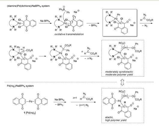
Scheme 5 The proposed mechanism for C1 polymerization of diazoacetates by the (diamine)Pd(0)(dichlone)/NaBPh<sub>4</sub> system.
