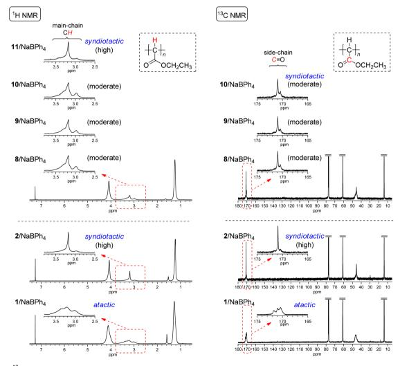
Fig. 4 <sup>1</sup>H and <sup>13</sup>C NMR spectra of polyEDA's obtained with 8/NaBPh<sub>4</sub> (run 5 in Table 2), 9/NaBPh<sub>4</sub> (run 8 in Table 2), 10/NaBPh<sub>4</sub> (run 12 in Table 2), and 11/NaBPh<sub>4</sub> (run 17 in Table 2), and with 2/NaBPh<sub>4</sub>, and 1/NaBPh<sub>4</sub>, recorded in CDCl<sub>3</sub> at 50 °C (<sup>1</sup>H NMR) or room temperature (<sup>13</sup>C NMR).
