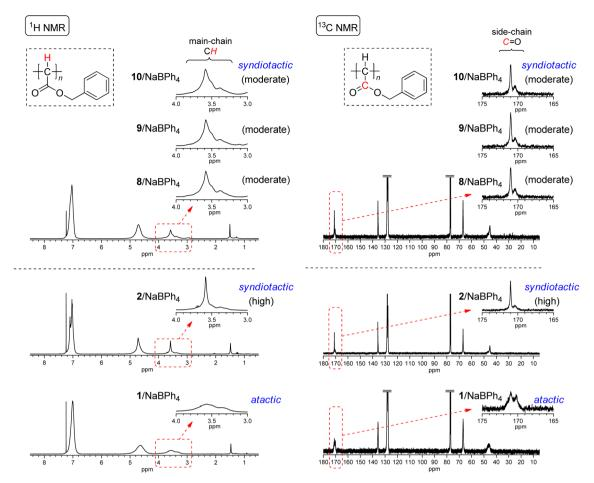
Fig. 6  $^{1}$ H and  $^{13}$ C NMR spectra of polyBDA's obtained with 2/NaBPh<sub>4</sub>, 1/NaBPh<sub>4</sub>, 8/NaBPh<sub>4</sub> (run 3 in Table 3), 9/NaBPh<sub>4</sub> (run 6 in Table 3), and 10/NaBPh<sub>4</sub> (run 7 in Table 3), recorded in CDCl<sub>3</sub> at 50  $^{\circ}$ C ( $^{1}$ H NMR) or room temperature ( $^{13}$ C NMR).
