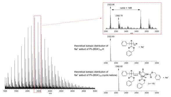
Fig. 5 MALDI-TOF-MS spectrum of polyBDA' obtained with the 10/NaBPh<sub>4</sub> initiating system ( $M_n = 5200$ , D = 2.24).
