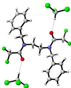
**Fig. 4** Single crystal X-ray structure of **3**, adopting conformation **3b'**. ( $\text{CHCl}_3$ )<sub>2</sub> stabilised by intermolecular  $\text{CF}_2\text{H}$ –phenyl interactions (see ESI Chapter 9†). The computed dipole moment is zero.
