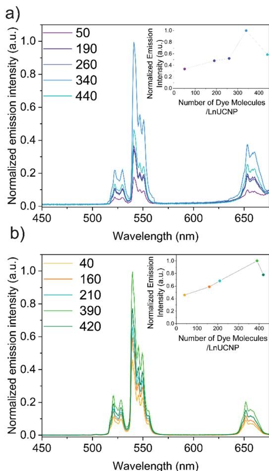
**Fig. 2** (a) Upconversion emission spectra of the SL system with different numbers of dye molecules per LnUCNP. (b) Upconversion emission spectra of the SE system with different numbers of dye molecules embedded into the silica shell per LnUCNP.
