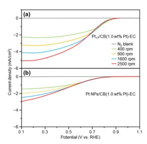
Fig. 5 Comparison of LSV curves of the samples. (a) Pt $_{17}$ /CB(1.0 wt% Pt)-EC. (b) Pt NPs/CB(1.0 wt% Pt)-EC. LSV curves were obtained for electrode rotation speeds of 400–2500 rpm under O $_2$  gas. Measurements under N $_2$  gas were conducted for baseline comparison. In these measurements, Pt loading was set to 0.204  $\mu$ g cm $^{-2}$ .
