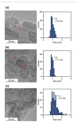
**Fig. 2** TEM images and histograms of each sample. (a)  $[Pt_{17}(CO)_{12}(PPh_3)_8]^2$ . (b)  $Pt_{17}(CO)_{12}(PPh_3)_8/CB$ . (c)  $Pt_{17}/CB$ . In (a), the parallel lines are not due to the lattice fringes of  $Pt_{17}$  cluster but due to the collodion membrane on the TEM grid.
