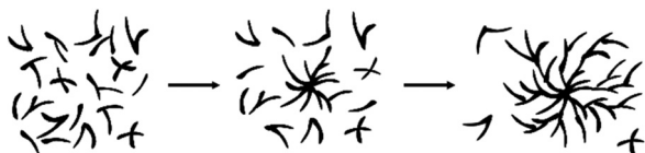
Scheme 2 Proposed mechanism for making polycrystalline nanodendrites. Nanopods form initially (left). Subsequent collisions result in branching of the arms in some nanopods, giving nanodendrites (middle). Continued collisions between nanopods and the arms of nanodendrites exhausts the supply of nanopods (right).
