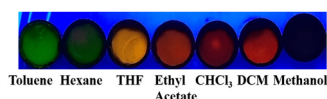
Fig. 10 The luminescence of BODIPY C1 on Whatman filter paper exposed to various solvent vapors taken under a UV lamp.
