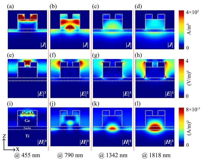
Fig. 3 Spatial xz-current density (|J|) (a-d), -electric field ( $|E|^2$ ) (e-h), and -magnetic field ( $|H|^2$ ) (i-l) distributions for a unit cell under TMpolarized light at wavelengths of 455 nm, 790 nm, 1342 nm, and 1818 nm. The dotted lines depict the proposed double grating absorber structure.
