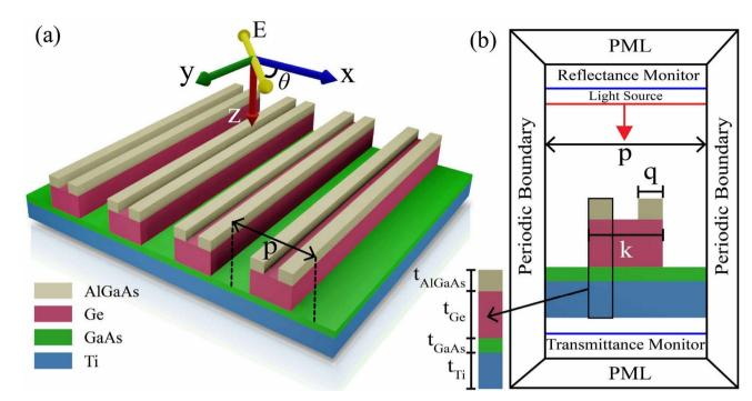
Fig. 1 (a) Illustration of a double-grating-based metamaterial absorber. A plane light wave was incident on the structure with an electric field along the z-direction where  $\theta$  is the polarization angle. (b) Cross-sectional view of the xz plane of our proposed absorber, where p=420 nm,  $t_{Ti}=200$  nm,  $t_{GaAs}=30$  nm,  $t_{GaAs}=3$
