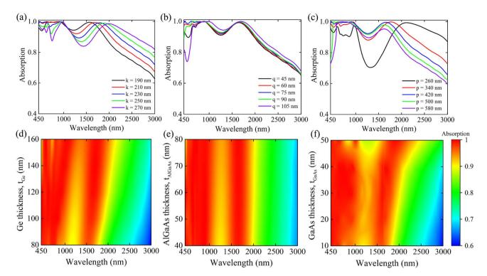
Fig. 4 Illustration of effects of the geometric parameters (a) k, (b) q, (c) p, (d)  $t_{Ge}$ , (e)  $t_{AlGaAs}$ , and (f)  $t_{GaAs}$  on absorption performances for TM-polarized light.
