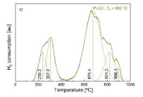
Fig. 6  $H_2$ -TPR curves of M-DCs produced at  $T_P = 600$  °C. Straight lines represent raw data, dashed lines the deconvoluted peaks and the corresponding maxima ((a) Ni-DC, (b) Cu-DC, (c) Pt-DC).
