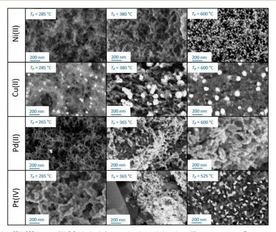
Fig. 4 Exemplary SEM-BSE images of M-DCs obtained after stopping the pyrolysis at three different temperatures  $T_{\rm P}$ .
