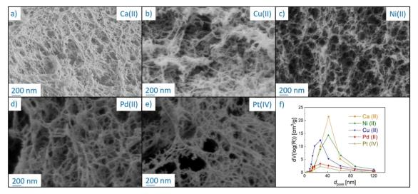
Fig. 1 (a)–(e) SEM pictures of inner pore structures of M-CAs crosslinked with different metal ions at  $c_m = 17$  mmol L<sup>-1</sup> and (f) their pore size distributions. Lines are drawn to guide the eye.
