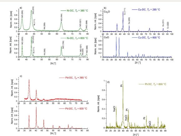
Fig. 5 XRD patterns of different metallic metal/metal oxide nanoparticles obtained from different M-Cas and different values of  $T_P$ : (a) Ni-DC, (b) Cu-DC, (c) Pd-DC, and (d) Pt-DC.
