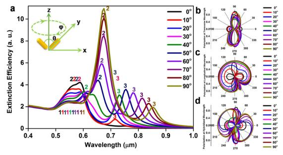
Fig. 2 Extinction and polarisation profiles (a) extinction spectra of gold nanorods dimers at different angular orientations calculated based on DDA technique; and (b-d) corresponding polarisation profiles at the wavelength maxima of the extinction profiles. The colour coded numerals 1, 2, 3 in panel a designate characteristic peaks for transverse, hybridised and longitudinal peaks at different angles of orientations.
