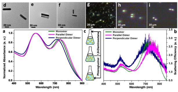
Fig. 1 Optical and structural characteristics (a) absorption and (b) scattering spectra of the monomeric and dimeric gold nanorods; (c) schematic depiction of the dimer formation from the monomeric building units upon addition of specific organic ligands; (d–f) transmission electron micrographs and (q–i) dark field microscopic images of the monomers and parallel and perpendicular dimers of gold nanorods.
