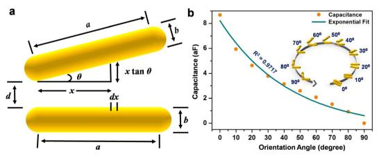
Fig. 6 Angle-resolved design of the capacitor (a) schematic illustration of the arbitrary formation of a capacitor with angular orientation of nanorod dimers; and (b) the exponential decay fit of the calculated values of the capacitance at different angular orientations of the gold nanorod dimers. The inset in panel b shows a schematic presentation of the gold nanorod dimer at different mutual orientations.
