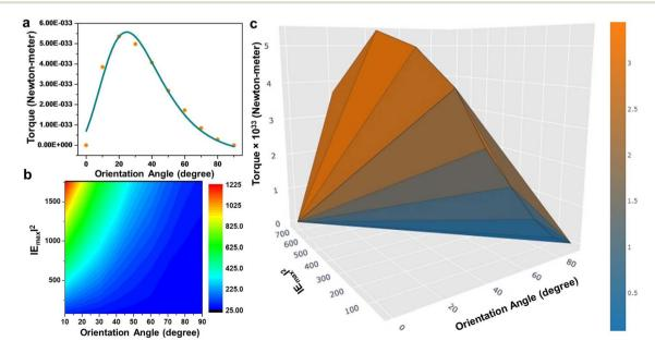
Fig. 5 Optomechanical characteristics (a) optical torque; and (b) electric field strength as a function of orientation angle of the gold nanorods; and (c) corresponding surface plot with the crest points twisted in xy-plane.
