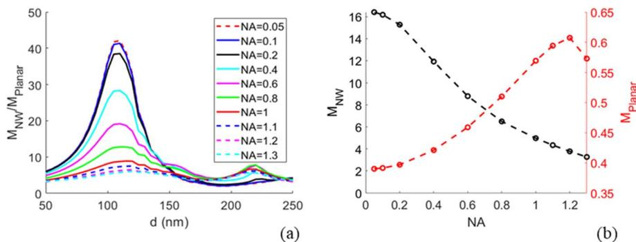
Fig. 5 (a) Modelled  $M_{NW}/M_{planar}$  for varying NA at  $\lambda = 640$  nm with  $L = 2$   $\mu\text{m}$  and  $t_{\text{oxide}} = 10$  nm. The simulations are performed with a step of 5 nm in  $d$ . Here,  $M_{planar}$  decreases from 0.57 to 0.39 as NA is decreased from 1.3 to 0.05. (b)  $M_{NW}$  and  $M_{planar}$  at varied NA for  $d = 110$  nm.
