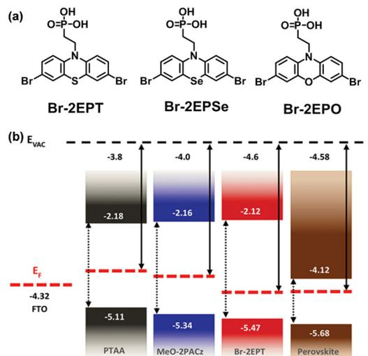
Fig. 6 (a) Molecular structures of Br-2EPT, Br-2EPSe, and Br-2EPO. (b) Energetic alignment of different SAMs and CsMAFA perovskite. Reproduced with permission.<sup>65</sup> Copyright 2022 Wiley-VCH GmbH.
