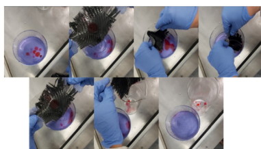
Fig. 13 Photographs outlining how coated carbon fibre supported by stainless steel mesh was utilised to remove silicone oil from the surface of water.
