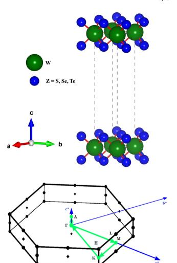
Fig. 1 The unit cell structure for  $WZ_2$  (Z = S, Se, and Te) materials and the BZ for the calculated band profiles.
