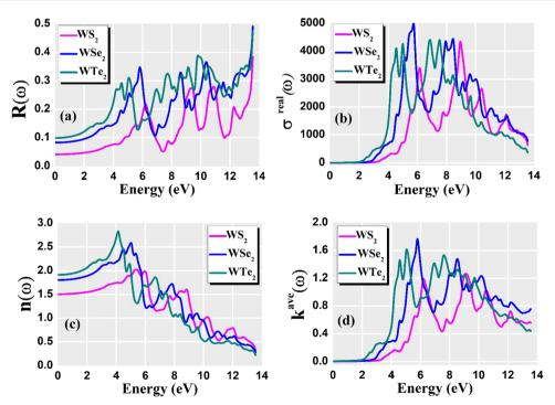
Fig. 7 The calculated frequency-dependent (a) reflectivity, (b) real part of optical conductivity, (c) refractive index, and (d) extinction coefficient for WZ<sub>2</sub> (Z = S, Se, and Te) materials.
