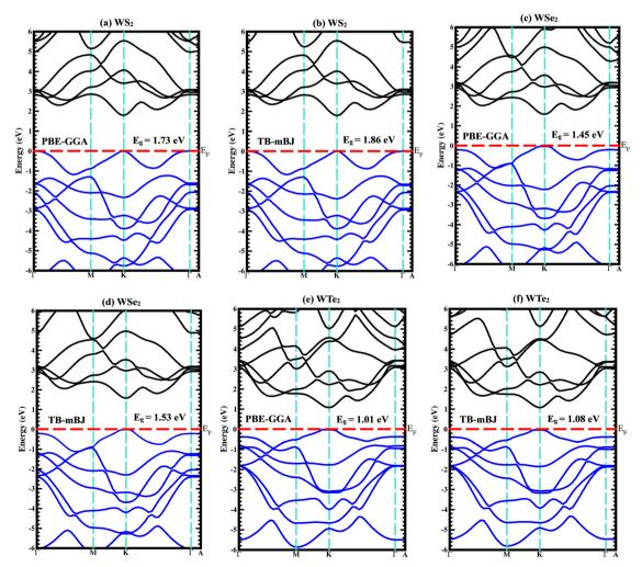
Fig. 4 Calculated band structures using both PBE-GGA and TB-mBJ potentials for (a), (b) WS<sub>2</sub>, (c), (d) WSe<sub>2</sub>, and (e), (f) WTe<sub>2</sub> materials.
