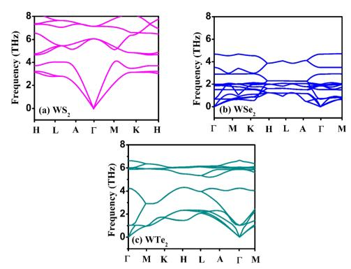
Fig. 2 The calculated phonon dispersion plots for the (a) WS<sub>2</sub>, (b) WSe<sub>2</sub>, and (c) WTe<sub>2</sub> materials
