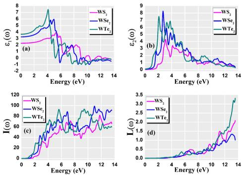
Fig. 6 The calculated frequency-dependent (a) real and (b) imaginary components of dielectric functions (c) absorption coefficients and (d) energy loss functions, for  $WZ_2$  (Z = S, Se, and Te) materials.
