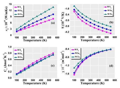
Fig. 8 Calculated (a) thermal conductivity, (b) Seebeck coefficient, (c) specific heat capacity, and (d) susceptibility of the  $WZ_2$  (Z = S, Se, and Te) materials.
