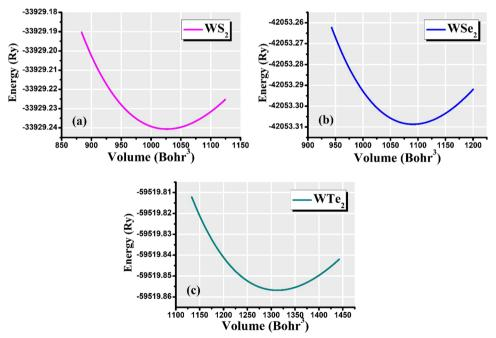
Fig. 3 Total-energy vs. volume optimization for the (a) WS<sub>2</sub>, (b) WSe<sub>2</sub>, and (c) WTe<sub>2</sub> materials.
