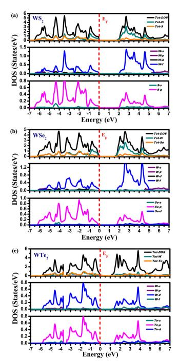
Fig. 5 The density of states for (a) WS<sub>2</sub>, (b) WSe<sub>2</sub>, and (c) WTe<sub>2</sub> materials.
