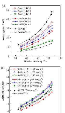
Fig. 5 (a) Water uptake and (b) the number of adsorbed water molecules per sulfonic acid group ( $\lambda$ ) for S-6H, S-6F, S-PPBP, and Nafion<sup>®</sup> 112 as a function of relative humidity at 80 °C.
