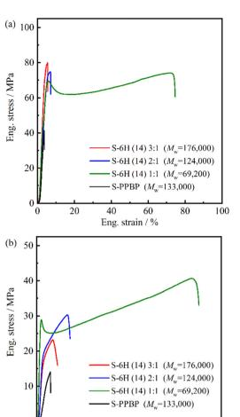
Fig. 7 Stress-strain curves of S-6H and S-PPBP acquired under (a) ambient conditions (RT, no extra humidification) and (b) at an elevated temperature and humidity (80 °C, 90% RH).
