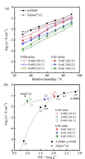
Fig. 6 (a) Proton conductivity of S-6H, S-6F, and S-PPBP as a function of relative humidity at 80 °C. (b) Relationship between proton conductivity and IEC of S-6H, S-6F, and S-PPBP-co-PPBP at 80 °C and 90% RH.
