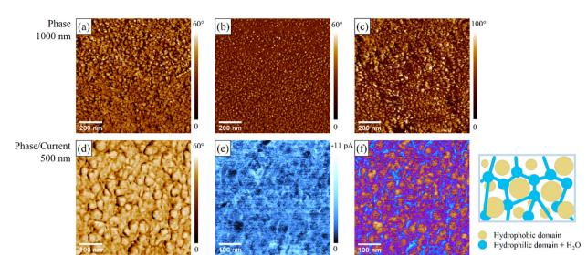
Fig. 8 e-AFM observations of S-6H membranes. Phase images of (a) S-6H (14) 3:1, (b) S-6H (14) 2:1, and (c) S-6H (14) 1:1 acquired under humid conditions (RT, 85% RH); scan size,  $1000 \times 1000$  nm<sup>2</sup>. (d) Phase (yellow coloured), (e) current-mapping (blue coloured), and (f) stacked images of S-6H (14) 3:1 obtained under ambient conditions; scan size,  $500 \times 500$  nm<sup>2</sup>.
