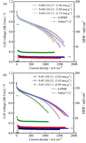
Fig. 11 IR-free cell voltage and HFR as a function of current density for a 5 cm $^2$ -sized PEFC with H $_2$  (500 mL min $^{-1}$ , 0.1 MPaG) and air (1000 mL min<sup>-1</sup>, 0.1 MPaG) feeds for (a) S-6H and (b) S-6F membranes at 80 °C and 100% RH.
