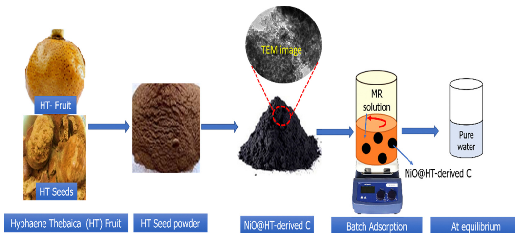
Fig. 1 Scheme for the preparation of the NiO@HT-derived C composite.
