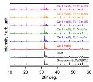
Fig. 1 XRD patterns of SCBO with and without emission ions.
