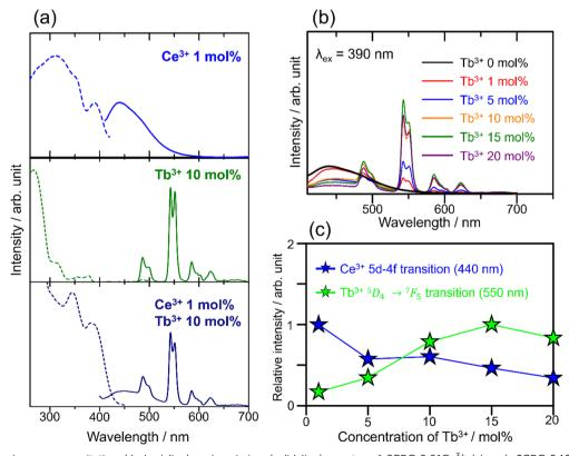
Fig. 5 (a) Photoluminescence excitation (dashed line) and emission (solid line) spectra of SCBO:0.01Ce<sup>3+</sup> (above), SCBO:0.10Tb<sup>3+</sup> (middle) and SCBO:0.01Ce<sup>3+</sup>, 0.10Tb<sup>3+</sup> (bottom). (b) Emission spectra of SCBO:0.01Ce<sup>3+</sup>, yTb<sup>3+</sup> (y = 0, 0.01, 0.05, 0.10, 0.15, 0.20) under 390 nm excitation and (c) relative emission peak intensities in 5d-4f (Ce<sup>3+</sup>; 440 nm) and  ${}^5D_4 \rightarrow {}^7F_5$  transitions (Tb<sup>3+</sup>; 550 nm).
