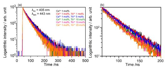
Fig. 6 (a) Photoluminescence decay curves of SCBO: $0.01Ce^{3+}$ ,  $yTb^{3+}$  (y = 0, 0.01, 0.05, 0.10, 0.15, 0.20) monitored 443 nm excited at 405 nm and (b) enlarged view of the decay curves between 60-200 ns.
