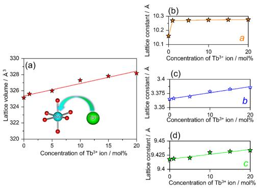
Fig. 4 Dependence of (a) the cell volume, lattice parameters, (b) a, (c) b, and (d) c on the concentration of Tb<sup>3+</sup> ion in SCBO:0.01Ce<sup>3+</sup>, yTb<sup>3+</sup> (y = 0, 0.01, 0.05, 0.10, 0.15, 0.20).
