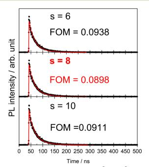
Fig. 7 Energy transfer analysis for SCBO: $0.01Ce^{3+}$ ,  $0.15Tb^{3+}$  by Inokuti–Hirayama model in s = 6 (above), s = 8 (middle) and s = 10 (bottom).
