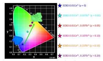
Fig. 8 Chromaticity diagram of SCBO:0.01Ce $^{3+}$ , yTb $^{3+}$  (y = 0, 0.01, 0.05, 0.10, 0.15, 0.20). Insert photographs show the blue-emitting SCBO:0.01Ce $^{3+}$  and green-emitting SCBO:0.01Ce $^{3+}$ , 0.15Tb $^{3+}$ .
