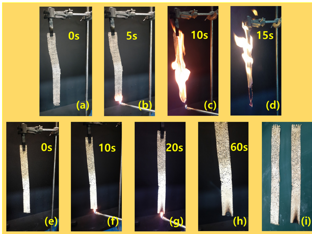
Fig. 8 Vertical burning tests of mHA-Jute bio-composites.
