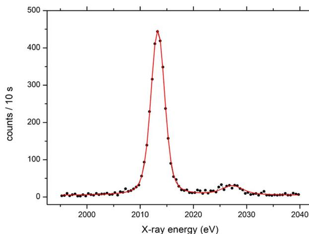
Fig. 7 P  $K\alpha$  spectrum of the NIST1573a reference standard containing  $2161 \pm 28 \text{ ppm}$  of phosphorus.
