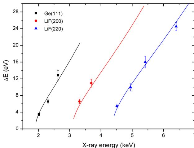
Fig. 6 Experimental energy resolution values determined from the fit of the model spectrum to the measured reference  $K\alpha$  spectra. The calculated energy resolution curves employing the divergence of the polycapillary lens are also plotted.
