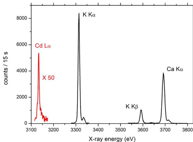
Fig. 9 PIXE spectrum of a *Noccaea praecox* powder pellet containing around 1300 ppm<sup>32</sup> of Cd recorded with the PB-WDS spectrometer. The spectrum was induced with 3 MeV protons; a beam current of 0.9 nA was used to scan the K and Ca energy range and it was increased to 3.8 nA during the scan over the Cd  $L\alpha$  range. Measured intensities of both scans were normalized to the proton dose measured with the beam chopper.
