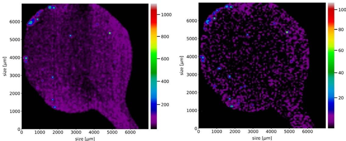
Fig. 10 Cadmium distribution maps in a *Noccaea praecox* leaf recorded with the PB-WDS spectrometer using the Cd  $L\alpha$  line (left), and the Si(Li) detector using the Cd K lines (right). The color scales represent measured counts.
