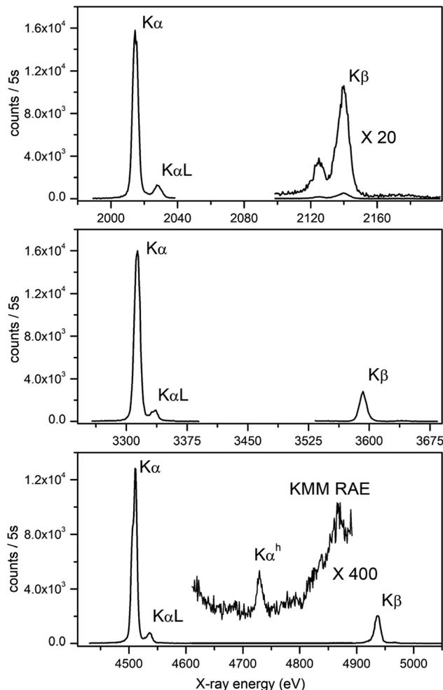
Fig. 4 Examples of high energy resolution proton induced X-ray spectra recorded with the PB-WDS spectrometer: P (top) and K spectra (middle) of a KH<sub>2</sub>PO<sub>4</sub> powder pellet recorded with Ge(111) and LiF(200) crystals, respectively, and the Ti spectrum (bottom) recorded with a LiF(220) crystal.
