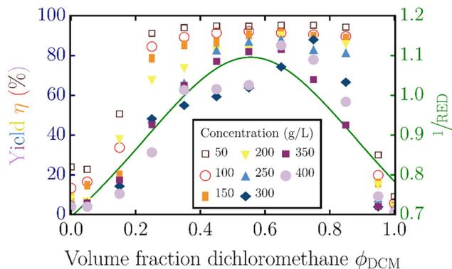
Fig. 5 Measured yield of the solubilized lignin (data points) and the inverse RED from the Hansen solubility parameters (green curve) as a function of the volume fraction of dichloromethane  $\phi_{DCM}$  in the dichloromethane–methanol solvent mixture. Experimental results in symbols reproduced from Yang *et al.*<sup>19</sup> Symbols and colors correspond to the different concentrations of lignin added to the solvent mixture.
