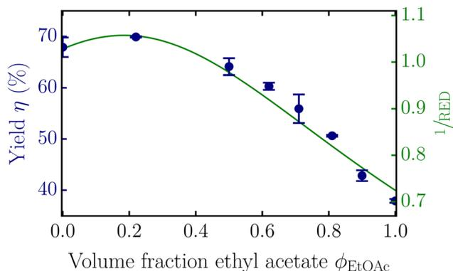
**Fig. 1** Measured yield of the solubilized lignin (data points) and the inverse RED from the Hansen solubility parameters (green curve) as a function of the volume fraction of ethyl acetate  $\phi_{\text{EtOAc}}$  in the ethyl acetate–methanol solvent mixture. The error bars indicate the standard deviations of duplicate experiments.
