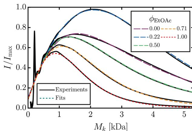
**Fig. 3** Examples of log-normal fits of eqn (3) to the molecular mass distribution of solubilized lignin fractions obtained at various solvent compositions as measured using GPC.  $I/I_{\max}$  is the normalized refractive index detector signal, which is proportional to the concentration (mass per unit volume).
