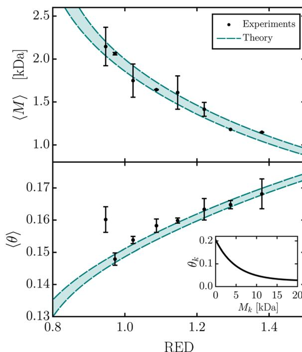
**Fig. 4** Weight-averaged molecular mass (top) and the fraction of functional groups (bottom) of the solubilized lignin fractions as a function of RED. These properties were measured experimentally (points) and predicted theoretically using eqn (5) and (6) (curves).
