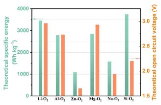
Fig. 1 The theoretical specific energy and open circuit voltage of various metal-air batteries. The specific energy is calculated by multiplying the theoretical specific capacity by the voltage.
