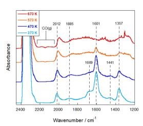
Fig. 5 In situ DRIFTS spectra under the RWGS reaction atmosphere over the Ru(col)/ZrTiO<sub>4</sub> catalyst without the electric field at 373-673 K; CO<sub>2</sub>:  $H_2: Ar = 1:1:2;$  40 SCCM total flow rate
