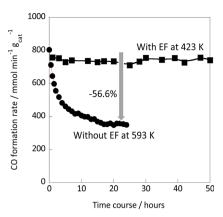
Fig. 3 Catalytic stability during the RWGS reaction over the Ru(col)/ $ZrTiO_4$  catalyst with/without the electric field (5 mA);  $CO_2: H_2: Ar = 1:1:2$ ; total flow rate: 100 SCCM; 100 mg catalyst weight.
