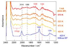
Fig. 6 In situ DRIFTS spectra under the RWGS reaction atmosphere over the Ru(col)/ZrTiO<sub>4</sub> catalyst recorded before/during application of the electric field (EF) at 423-573 K;  $CO_2: H_2: Ar = 1:1:2$ ; 40 SCCM total flow
