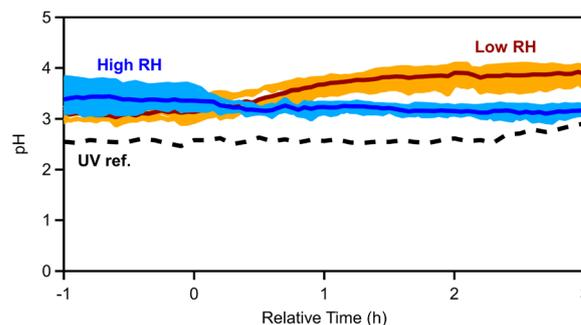
Fig. 8 Estimated aerosol pH for all dark experiments (light blue shaded regions correspond to the variability across the high RH, while orange corresponds to the dry experiments, with solid blue and red lines being the median across the RH and dry experiments, respectively) and dashed black lines correspond to the UV reference experiment.
