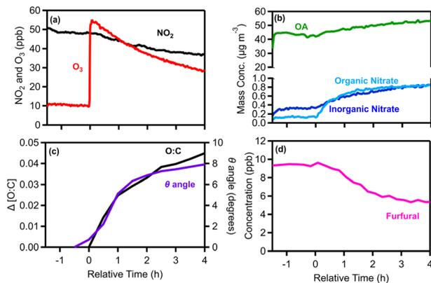
Fig. 4 Measurements for experiment 1 (typical dark oxidation experiment) showing (a)  $\text{NO}_2$  and  $\text{O}_3$ , (b) wall-loss corrected OA, particulate inorganic and organic nitrate, (c) the change in the O : C ratio and theta angle and (d) furfural;  $m/z$  97.
