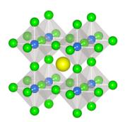
Fig. 1 Crystal structure of alkali metal rich antiperovskite  $M_3BTe$  (M=Li, Na, K; B=H, F). The newly synthesized  $K_3HTe$  and  $K_3FTe$  adopt the cubic symmetry ( $Pm-\bar{3}m$ ). The B-site anion (H or F) (blue) occupies the octahedral center formed by K cations (green) and the A-site telluride anion (yellow) occupies the cuboctahedral site.
