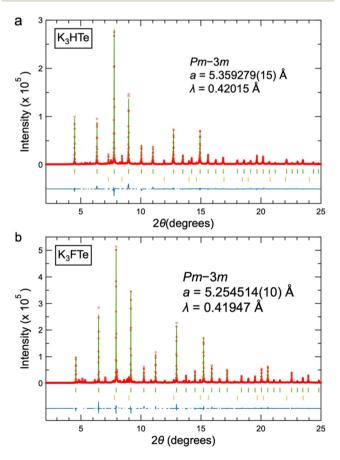
**Fig. 2** Rietveld refinement of SXRD data of (a)  $K_3HTe$  and (b)  $K_3FTe$ . The red circles, the green solid line, and the blue solid line represent the observed, calculated, and difference intensities, respectively. The upper ticks indicate the calculated Bragg reflections for (a)  $K_3HTe$  and (b)  $K_3FTe$ , while the lower ticks for (a) KH and (b) KF. The unknown peaks are removed from the refinement.
