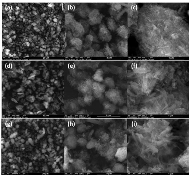
Fig. 10 SEM images at different magnifications of water-free  $\text{Zn}_x\text{Co}_{1-x}\text{Al}$  oxides: (a–c)  $x = 0$ ; (d–f)  $x = 0.2$ , and (g–i)  $x = 0.4$ .
