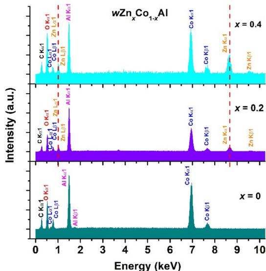
Fig. 11 EDX spectra of water-added  $w\text{Zn}_x\text{Co}_{1-x}\text{Al}$  oxide powders ( $x = 0, 0.2, 0.4$ ).
