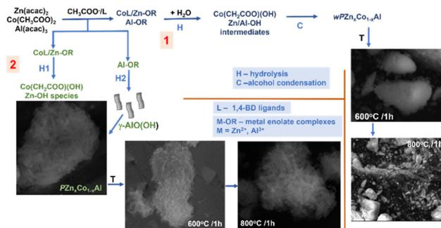
Scheme 1 Possible reaction pathways for the formation of water-assisted,  $wPZn_xCo_{1-x}Al$ , and water free precursors,  $PZn_xCo_{1-x}Al$ , and of their corresponding calcination products,  $wPZn_xCo_{1-x}Al$  and  $Zn_xCo_{1-x}Al$ .
