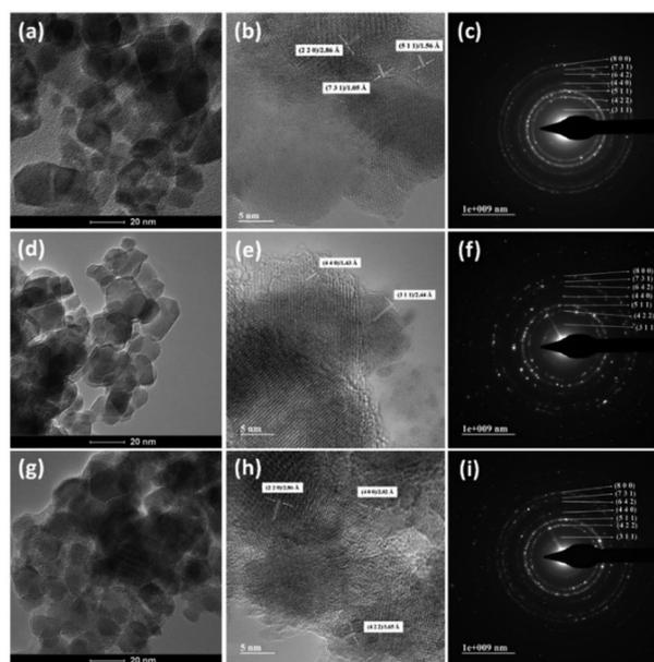
Fig. 13 (a), (d) and (g) TEM images; (b), (e) and (h) HRTEM images and (c), (f) and (i) SAED patterns of the water-added  $w\text{Zn}_{1-x}\text{Co}_x\text{Al}$  powders: (a)–(c)  $x = 0$ ; (d)–(f)  $x = 0.2$  and (g)–(i)  $x = 0.4$ .
