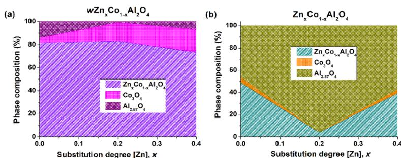
Fig. 3 Chart diagrams showing the variation of the phase composition depending on the zinc substitution degree ( $x$ ) for: (a) water-assisted  $w\text{Zn}_x\text{Co}_{1-x}\text{Al}$  and (b) water-free  $\text{Zn}_x\text{Co}_{1-x}\text{Al}$  oxides.
