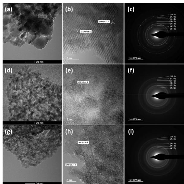
**Fig. 14** (a), (d) and (g) TEM images; (b), (e) and (h) HRTEM images and (c), (f) and (i) SAED patterns of the water-free  $Zn_{1-x}Co_xAl$  powders: (a)–(c)  $x = 0$ ; (d)–(f)  $x = 0.2$  and (g)–(i)  $x = 0.4$ .
