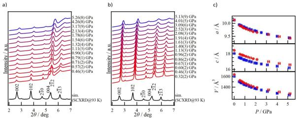
Fig. 6 Variable-pressure PXRD measurements for (a) 2 and (b) 3 in the range of  $1.0 \times 10^{-4}$  (1 atm) -5.26 and  $1.0 \times 10^{-4}$  (1 atm) -5.13 GPa, respectively. Simulation curves (black line) were derived from the SCXRD results at 93 K. (c) Pressure dependence of cell parameters (top) a, (middle) c and (bottom) V for 2 (red circles) and 3 (blue squares). The black filled circle and square represent the simulation derived from the SCXRD results at 93 K for 2 and 3, respectively.
