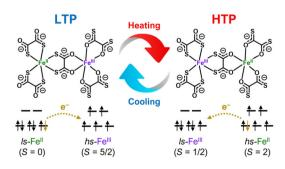
Fig. 1 A charge-transfer phase transition (CTPT) model of 1.
