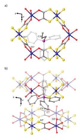
Fig. 2 (a) Coordination environment of O<sub>6</sub> and S<sub>6</sub> atoms for the two Fe ions in 3. Colour codes: gray, red, yellow, purple and navy represent C, O, S, P, and Fe atoms, respectively. A 2-D honeycomb layer in the ab plane is shown. (b) Layered structure along the c axis. One side of two disordered configurations is shown in the "PrPh3P position. Symmetry codes: (a) 1+x, 1+y, +z; (b) 1+y, 1-x+y, 1/2+z; (c) 1-y+x, +x, 1/2+z.
