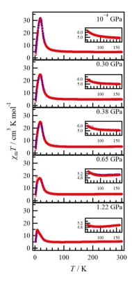
Fig. 3 Temperature dependence of the product,  $\chi_m T$ , measured at 5 kOe for 3. Red open and blue filled circles represent the heating and cooling processes, respectively, under  $1.0 \times 10^{-4}$ , 0.30, 0.38, 0.65 and 1.22 GPa. The inset shows a magnified plot.
