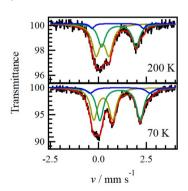
Fig. 5  $^{57}$ Fe Mössbauer spectra of (a) 2 and (b) 3 at 70 and 200 K (black lines). Yellow doublets represent the ls-Fe $^{II}$  ion and the blue and green lines represent the hs-Fe $^{II}$  ion. Red lines are the sum of the above three simulated lines.
