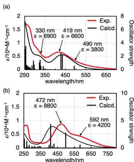
**Fig. 3** UV-vis absorption spectra (red lines) of (a) **1** ( $1.1 \times 10^{-3}$  M) and (b) **2** ( $4.0 \times 10^{-5}$  M) in CHCl<sub>3</sub> (293 K), along with the computed spectrum of V(O)XL (black lines) at the B3LYP/Def2SVP (PCM: CHCl<sub>3</sub>) theoretical level.
