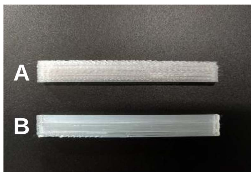
Fig. 5 Examples of impact test samples with different qualities: under-extruded (A) and close to the ideal weight (B).
