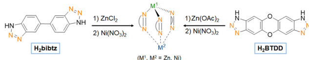
Fig. 10 Representation of how the H 2 bibtz (1 H ,1' H -5,5'-bibenzof[ d ][1,2,3]triazole) linker and the H 2 BTDD linker, used respectively to synthesize CFA-1 and MFU-4l enable to obtain the same scorpionate-like configuration with three coordinating nitrogen atoms embedded within the MOF structure.
