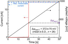
Fig. 3 Typical current response of a BLM under linearly rising membrane voltage.  $\Delta\psi_{\rm appl,C}$  denotes the critical applied voltage for membrane breakdown. The mean value of  $\Delta\psi_{\rm appl,C}$  is indicated on the figure.
