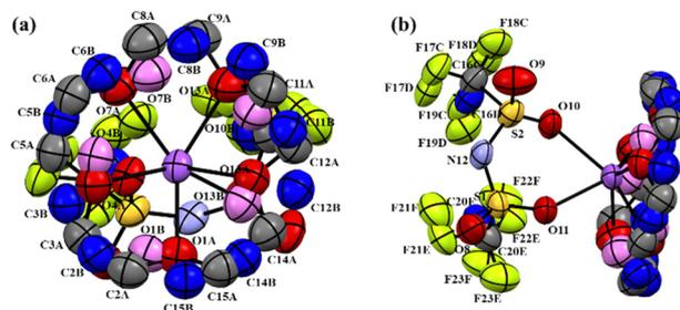
Fig. 9 ORTEP representation of [Na 15C5] at 253 K temperature where the disordered parts A and B occupancy were 72% and 28%, respectively. The low occupancy part of the disordered molecules carbon, oxygen and fluorine are coloured as blue, violet and green, respectively. Hydrogens are omitted for clarity.
