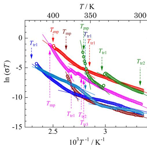
Fig. 10 Arrhenius plots of electrical conductivity. [Li 12C4] (○), [Na (12C4)<sub>2</sub>] (○), [Li 15C5] (○), [Na 15C5] (○), [K (15C5)<sub>2</sub>] (○), and [Na 18C6] (○).
