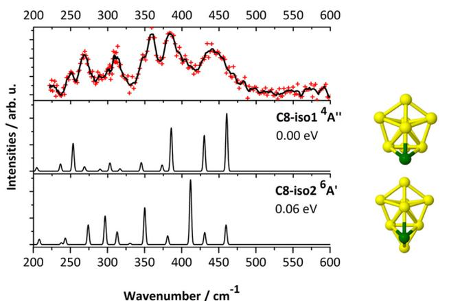
Fig. 4 IR-MPD spectrum of CrSi<sub>8</sub><sup>+</sup>·Ar (upper panel) and calculated harmonic infrared spectra (B3P86/6-311+G(d)) of low-energy isomers of CrSi<sub>8</sub><sup>+</sup>.
