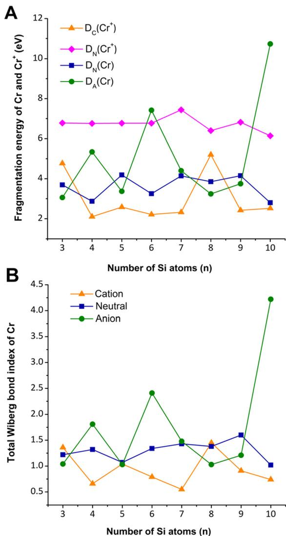
Fig. 8 Fragmentation energy to remove either Cr or Cr<sup>+</sup> (A) and total Wiberg bond index of Cr (B), in the lowest-energy cationic, neutral and anionic lowest-lying CrSi<sub>n</sub><sup>+0/-</sup> isomers with *n* = 3–10. Calculated values are obtained from B3P86/6-311+G(d) + ZPE computations.
