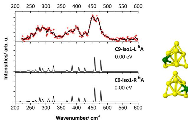
Fig. 5 IR-MPD spectrum of CrSi<sub>9</sub><sup>+</sup>·Ar (upper panel) and calculated harmonic infrared spectra (B3P86/6-311+G(d)) of low-energy isomers of CrSi<sub>9</sub><sup>+</sup>.
