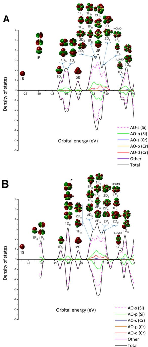
Fig. 7 Calculated density of states (DOS) of cationic  $\text{CrSi}_{10}^+$  (A) and neutral  $\text{CrSi}_{10}$  (B) and the projection of the DOS onto atomic orbitals (AO) of Si and Cr. Positive and negative DOS represent spin-up and spin-down electrons, respectively.
