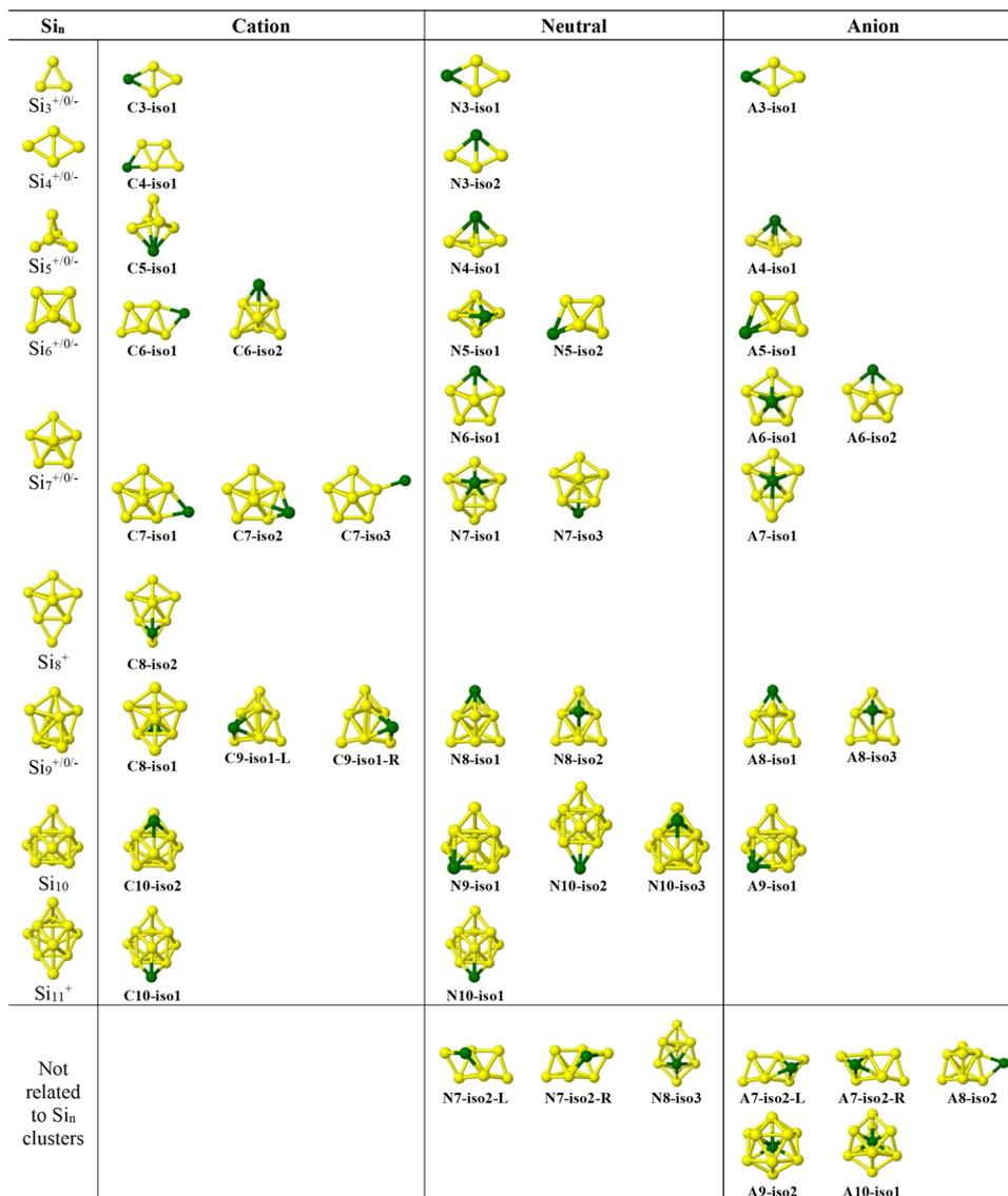
Fig. 1 Diagram illustrating the structural evolution of cationic, neutral and anionic chromium doped silicon clusters in comparison with the pure silicon clusters. Structures of cationic, neutral, anionic pure silicon clusters are taken from ref. 42–44, 67, 70–73 and re-calculated at the B3P86/6-311+G(d) level.
