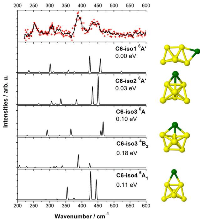
Fig. 2 IR-MPD spectrum of  $\text{CrSi}_6^+\cdot\text{Ar}$  (upper panel) and simulated harmonic infrared spectra of low-energy isomers of  $\text{CrSi}_6^+$  (B3P86/6-311+G(d)). Geometric structures of the low-energy isomers are shown on the right. Experimental data points are shown as red crosses, while the full black line corresponds to a three-point running average.
