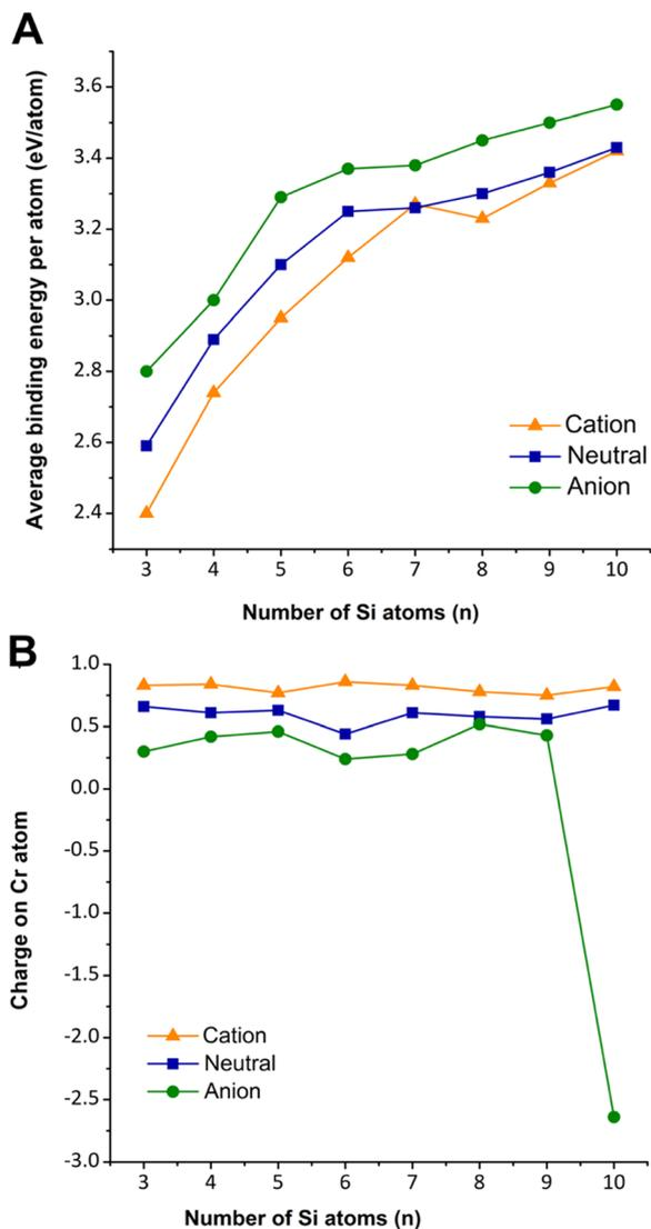
Fig. 10 Average binding energy per atom (A) and charges on Cr atom (B), in the lowest-energy cationic, neutral and anionic lowest-lying  $\text{CrSi}_n^{+0/-}$  isomers with  $n = 3-10$ . Calculated values are obtained from B3P86/6-311+G(d) + ZPE computations.
