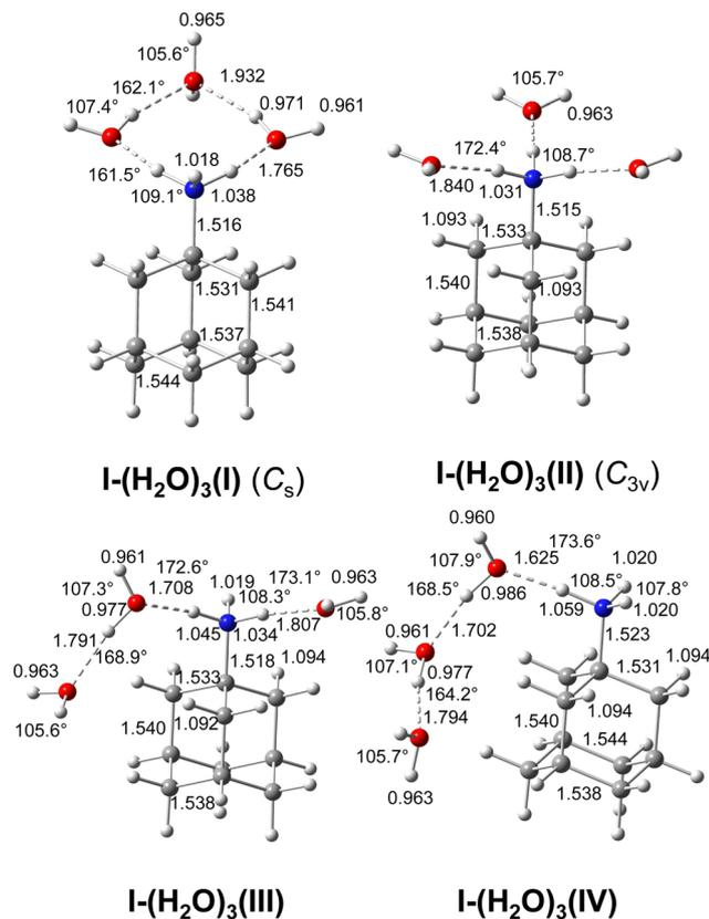
Fig. 6 Calculated equilibrium structures (in Å and degrees) of **AmaH<sup>+</sup>(I)(H<sub>2</sub>O)<sub>3</sub>(I-IV)** in their ground electronic state (B3LYP-D3/cc-pVTZ). All bond lengths are shown in ESI† (Fig. S24).
