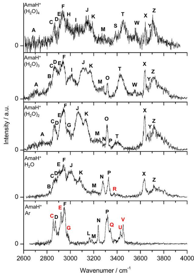
Fig. 2 IRPD spectra of AmaH<sup>+</sup>(H<sub>2</sub>O)<sub>*n*</sub> (*n* = 1–4) in the 2600–4000 cm<sup>-1</sup> range recorded in the H<sub>2</sub>O loss channel are compared to the IRPD spectrum of AmaH<sup>+</sup>Ar.<sup>49</sup> The position, widths, and assignments of the transitions observed (A–Z) are listed in Table 1. The bands that can only be assigned to the iminium isomers are highlighted in red.
