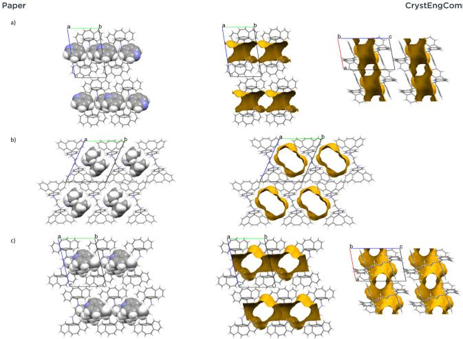
Fig. 1 Unit cells (left) and void diagrams (right) for a)  $H1\cdot 2(PYR)$ , b)  $H1\cdot 2(2MP)$  and c)  $H1\cdot 2(4MP)$ .
