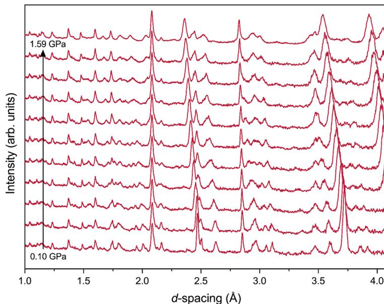
Fig. 6 Neutron powder-diffraction patterns of TFE obtained from PEARL, collected at 200 K, shown with increasing pressure (form 1 – red).
