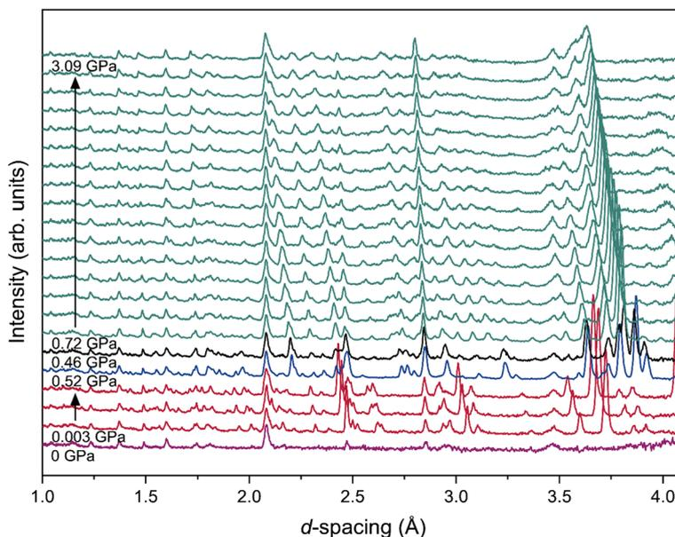
Fig. 5 Neutron powder-diffraction patterns of TFE obtained from PEARL, collected at 245 K, shown with increasing pressure (liquid – purple; form 1 – red; form 2 – blue; form 3 – cyan; mixed phase of forms 2 and 3 – black).
