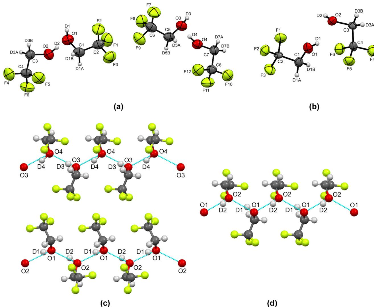
**Fig. 2** The labelling scheme used for the high-pressure single-crystal X-ray diffraction structures of TFE (a) form 3 [295(2) K; 0.71(5) GPa] and (b) form 4 [295(2) K; 2.09(5) GPa], with thermal ellipsoids drawn at the 50% probability level. The hydrogen-bonded chains formed are shown in (c) form 3 and (d) form 4, where the hydrogen bonds are represented by light-blue dashed lines (C – dark grey, H – light grey, O – red, F – green).
