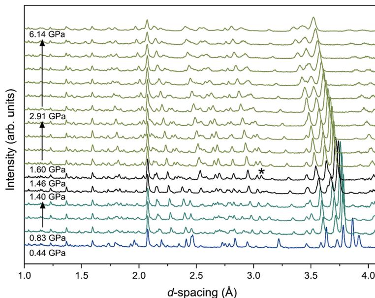
Fig. 1 Neutron powder-diffraction patterns of TFE obtained from PEARL, collected at 295 K, shown with increasing pressure. The peak at  $\sim 3.06 \text{ \AA}$  corresponding to the (112) reflection in form 4 is shown by \* (form 2 – blue; form 3 – cyan; form 4 – green; mixed phase of forms 3 and 4 – black).
