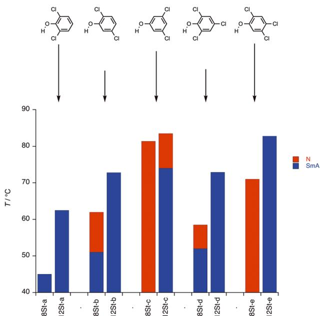
**Fig. 12** Comparison of the mesophase transition temperatures for the new complexes in this study. Note that melting points are not shown and that, with the exception of the data for 12St-c, all temperatures are monotropic. Melting points have not been indicated in the plot.
