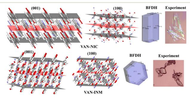
Fig. 3 Crystal morphologies and molecular packing of the (001) and (100) faces of vanillin-nicotinamide (VAN-NIC) and vanillin-isonicotinamide (VAN-INM).
